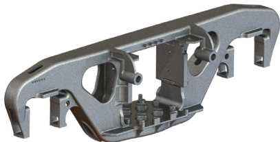
Side frame of the freight car bogie with an axial load of 25 tf
